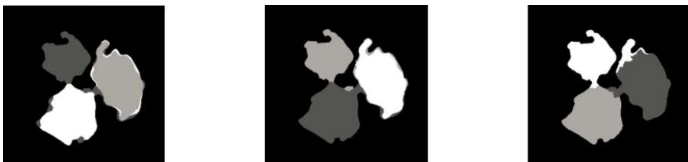
Figure 5: Results of k-means clustering and morphological hole-filling, with variation of the spatial weighting parameter for feature extraction. From left to right, the values of the parameter are: a) 0.05, b) 0.4 (ideal), and c) 2.0.
