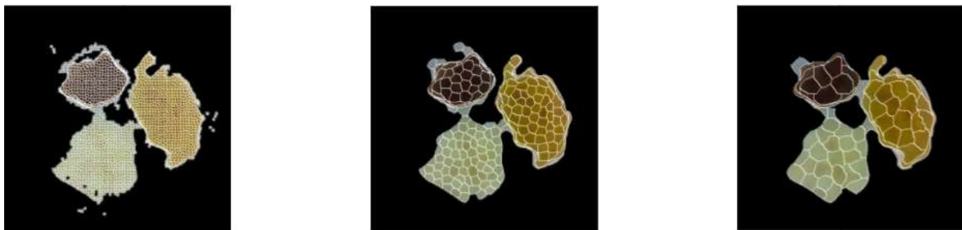
Figure 3: Results of superpixel segmentation, with variation of the region size parameter with a constant spatial regularization parameter of 0.01. From left to right, the values of the parameter are: a) 5, b) 15 (ideal), and c) 25.
