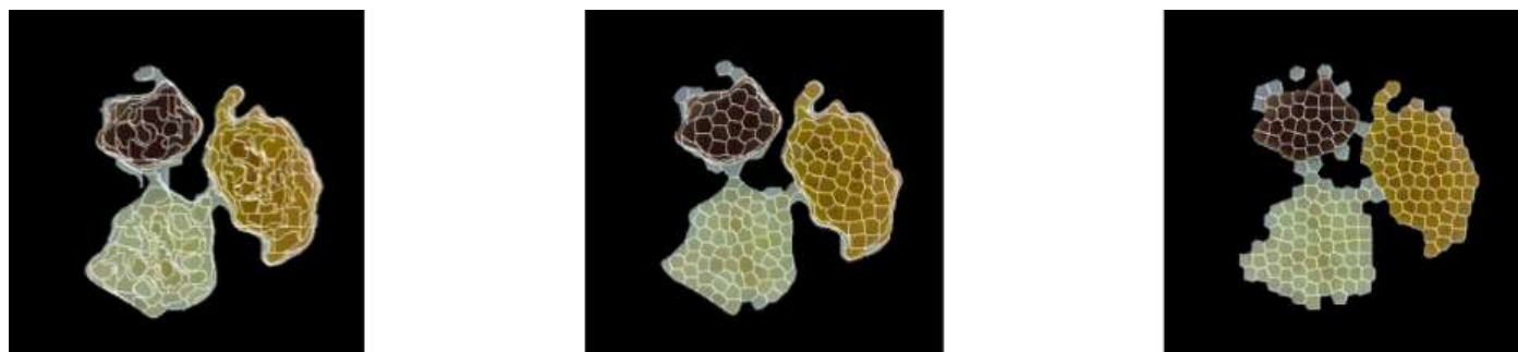
Figure 4: Results of superpixel segmentation, with variation of the spatial regularization parameter with a constant region size parameter of 15. From left to right, the values of the parameter are: a) 0.0001, b) 0.01 (ideal), and c) 1.
