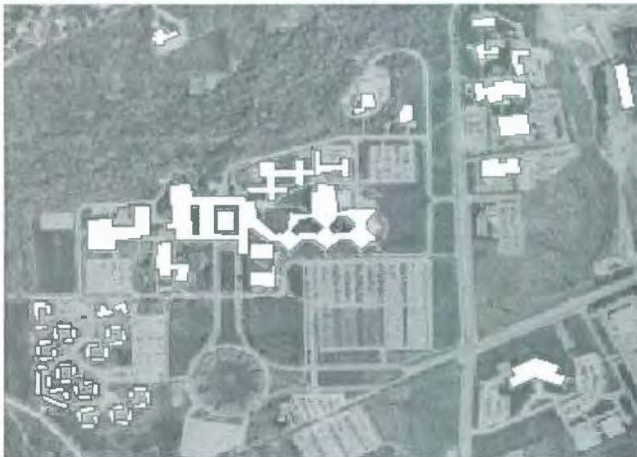
Figure 5. Building footprints added using "head's up digitizing".
