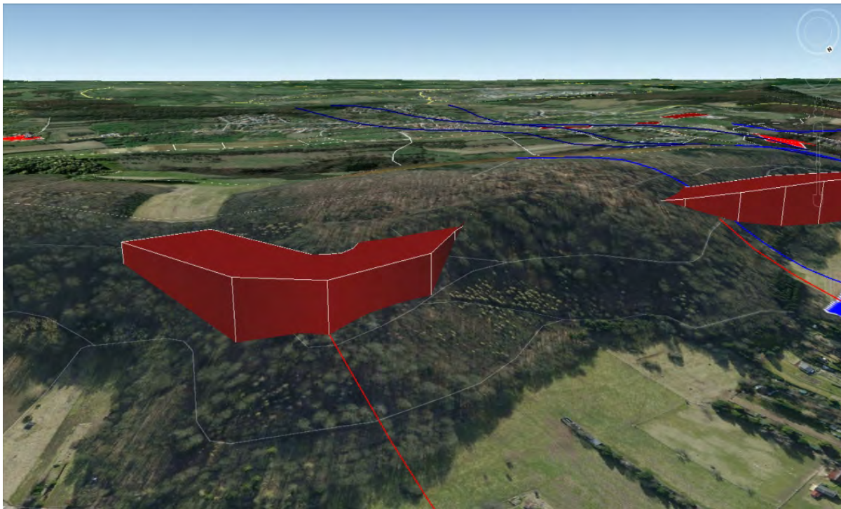
Figure 4. Notice in the middle how the polygon disappears, and on the left extends longer than 2m. This is a problem with Google Earth's "Relative to ground" option when using small polygon heights.
