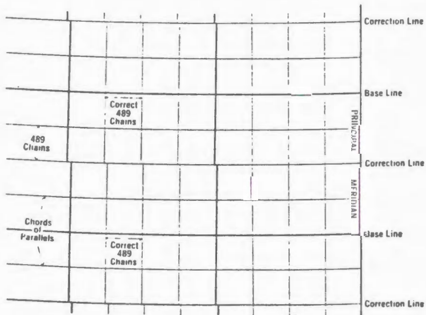
Figure 1b : The Dominion Land Survey system of townships. In this system the standard width of a township is 489 chains (i.e. six miles plus six road allowances of 1.5 chains).
