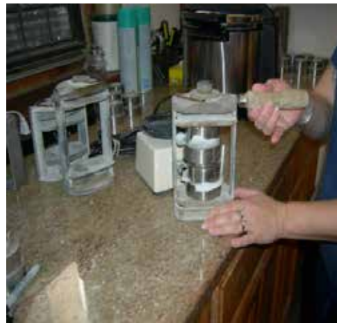
Figure 8. Use of Carver press to remove air from custom prosthesis prior to hardening.
