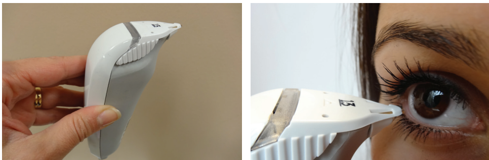
Supplementary Figure 2. TearLab osmometer handle and tear sampling from lower temporal tear meniscus.
