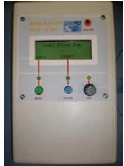
Figure 2: The control box sets temperature, purge and refill times, and the amount of time lenses are in and out of the fluid bath.
