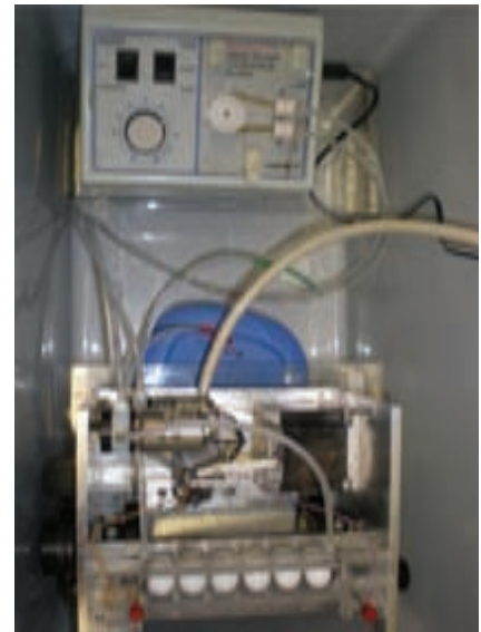
Figure 1: The model blink cell, showing the pistons, valves, tubing series, pump and sensors
