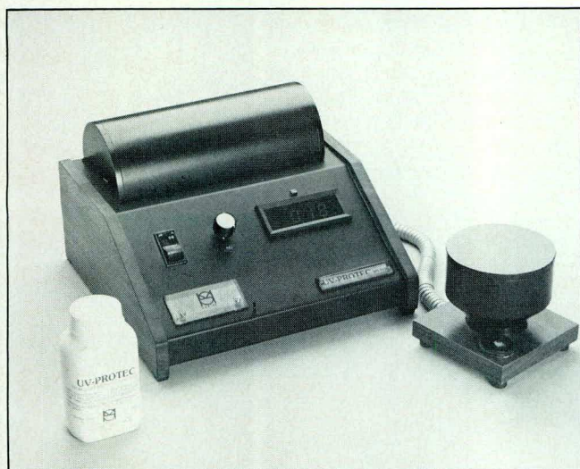
Fig. 1 Prototype UV-PROTEC meter. The current production model does not use the separate sensing unit illustrated to the right of the meter.
