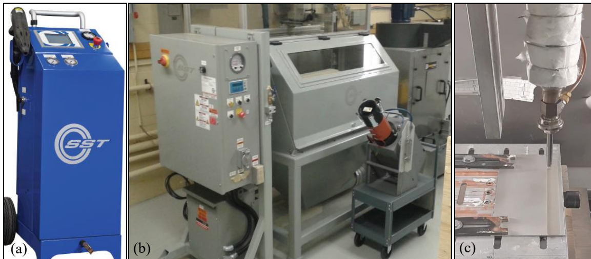
Figure 1: (a-b) SST Series P cold spray system with pressure, control, powder feeder, spray booth, and dust collector units, (c) the cold spray gun and nozzle during Ni-coating process of samples.
