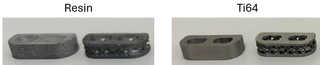
Figure 2. Left: Resin printed implants (flat-solid and flat-latticed). Right: Ti64 printed implants (flat-solid and flat-latticed).
