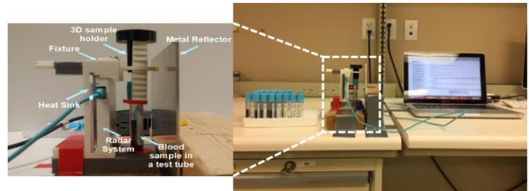
Fig. 1: The experiment setup showing the integrated radar system connected to PC interface where the collected raw data are monitored and processed using DSP algorithms for accurate identification
