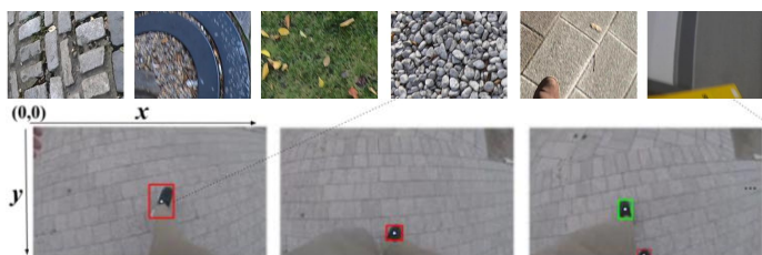
Fig. 1: Machine learning methods have been developed by our team to (A) identify different surfaces captured in indoor and outdoor environment (upper panel) and (B) estimate pixel-wise spatiotemporal gait parameters by localizing feet in 2D coordinate system of the frames captured by a belt-mounted camera (lower panel).
