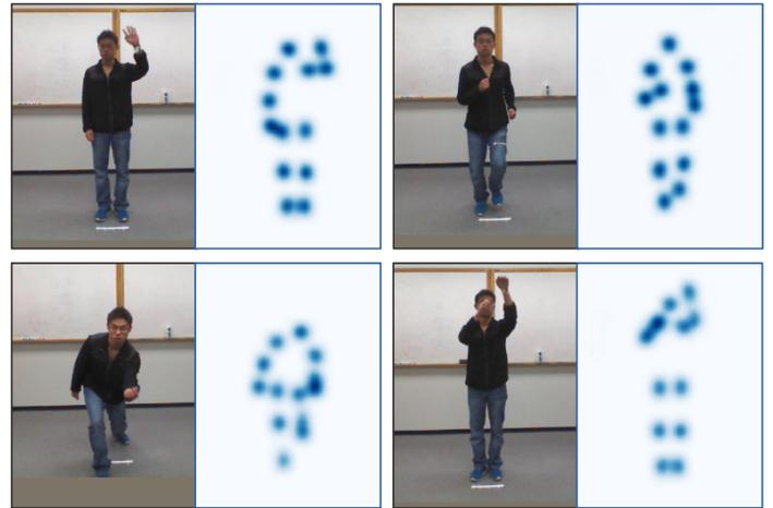
Fig. 1: Spatial slices of compressed spatio-temporal pose encodings. The spatial fusion compresses the pose information, enabling it to be processed by a standard CNN classifier. Sample images taken from the *wave*, *jog*, *bowling*, and *basketball shot* classes of UTD-MHAD [10].
