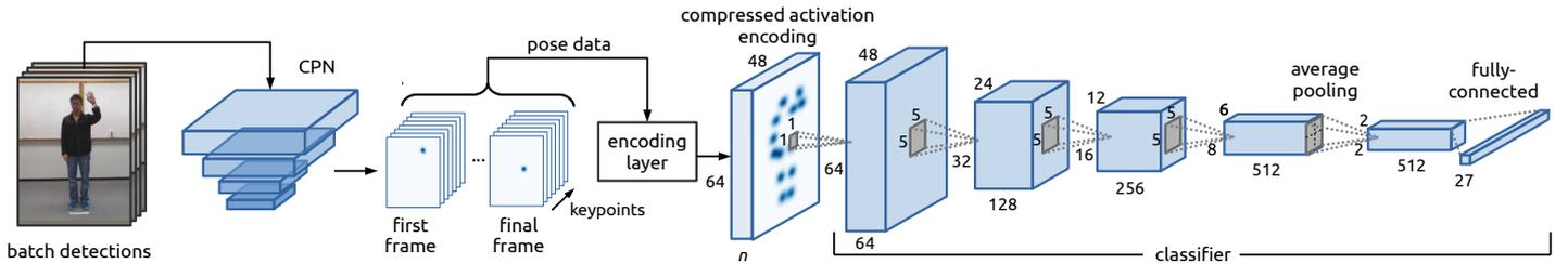
Fig. 2: Proposed action recognition model. The classifier takes as input the compressed spatio-temporal pose encodings and includes four convolutional layers, an average pooling layer, and a final fully-connected layer.
