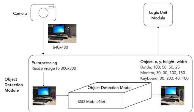
**Fig. 2: Object detection module overview.** Once the camera takes a snapshot of the scene, the image is passed to the object detection module. First, preprocessing is done, such as re-sizing the image to 300x300. Then, the preprocessed image is sent to an object detection model where the most probable object type and bounding box of each object are determined for each object. The object types and corresponding bounding boxes are then sent to the logic unit module.
