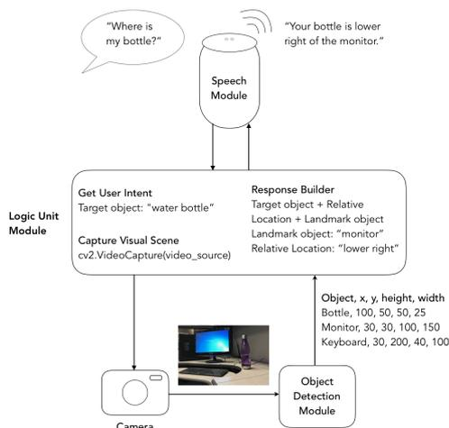
Fig. 3: Logic unit module. First, the user request gets processed, then the camera command is executed. After the image is processed by the object detection module, the types and locations of each object identified are sent to the response builder. The response builder finds the closest landmark object to the object of interest based on the user’s intent, calculates the relative location, and builds the user response. Lastly, the response is communicated to the user via the speech module.
