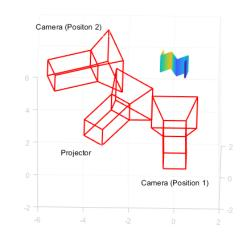
Fig. 1: Moving-Camera and Projector for Non-Planar Scene
