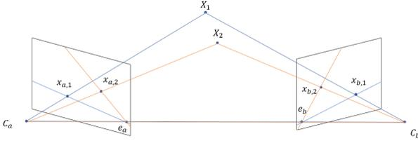
Fig. 2: Epipoles ( $e_j, C_j$ )  $j = a, b$  connect camera centers  $C_j$  and the intersection of line  $(C_a, C_b)$  and image planes at  $e_j$ . These epipoles connect any observed image point  $x_a$ , 3D coordinate  $X$  and corresponding image point  $x_b$  over a set of epipolar lines  $\{(x_a, e_a), (x_b, e_b)\}$  from which geometric understanding of the scene can be constructed.
