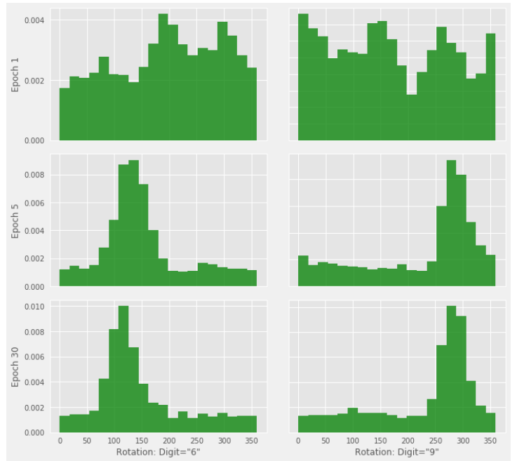
Fig. 5: Evolution of rotations encoded by the AVAE during training. Distribution of rotations of the "6" and "9" digits during training of the AVAE at epochs 1, 5 and 30. As training progresses the AVAE learns to encode most digits at the same orientation, but additionally these numbers are encoded as 180^\circ rotations of one another.
