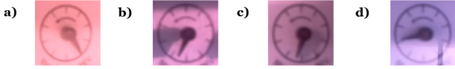
Fig. 2: a) A sample cropped image with no artifact, b) with heavy shadow, c) blurry due to windy condition, and d) glare due to direct sunbeam reflection.
