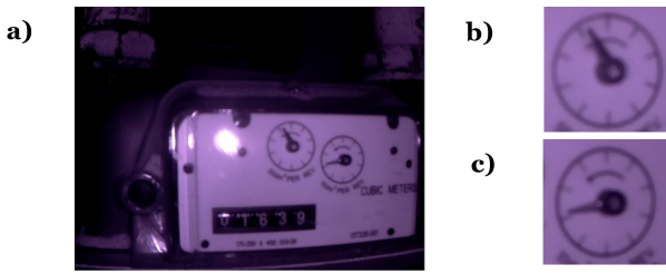
Fig. 1: a) A sample raw image of the gas meter panel captured at night, b) cropped image of the respective left dial, and c) cropped image of the respective right dial.
