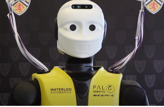
Fig. 1: REEM-C Humanoid Robot, with RGB-D camera shown on forehead
