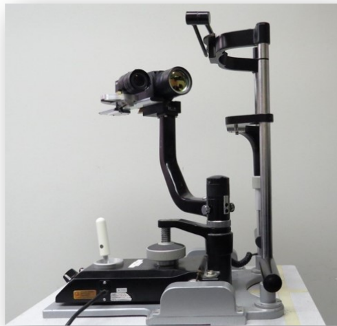
Fig. 1: The ThermOcular device used for Ocular Surface Temperature assessment.[1]
