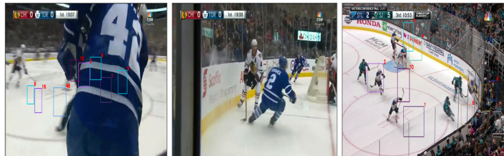
Fig. 1: MHPTD failure modes: L-R (Erroneous, Missing & Offset) bounding boxes,
