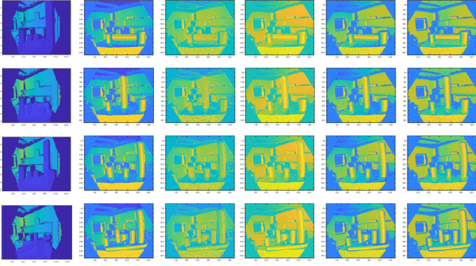
(a) I_\theta images of the estimation results of different algorithms (Real images). From left: the depth map, the normals ground truth, Fan's method [19], Nakagawa's method [18], Moradi's method [20], the proposed method.
