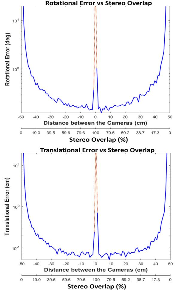
Figure 2: Error plots for Study 1. Errors generally increase as stereo overlap decreases. At 100% overlap, close camera placement causes numerical instability, indicated by red dotted lines.
