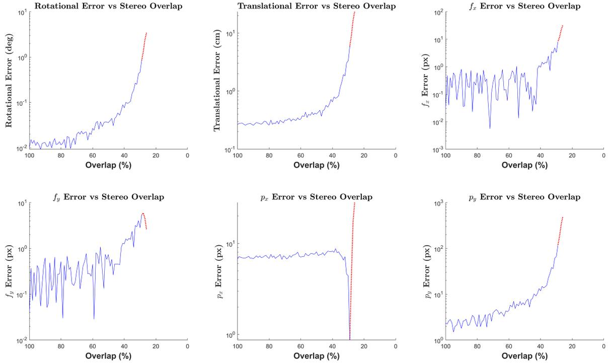
Figure 3: Error plots for Study 2. Errors increase as stereo overlap decreases, with red dotted lines marking reprojection errors exceeding 3 pixels, where calibration accuracy becomes unacceptable. Calibration is not computed below 20% overlap due to insufficient correspondences.
