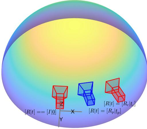
Figure 1: Simulation setup with red representing cameras and blue representing projector, all projecting onto the hemispherical surface.
