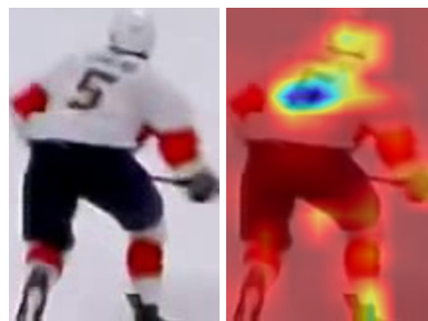
Figure 2. OSNet activation map. A player frame is shown alongside the corresponding OSNet final layer activation map. The network focuses on the jersey number region, which indicates that OSNet learns the importance of jersey number even without explicit supervision.
