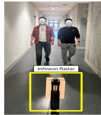
Figure 2. Experiment setup for 2 people walking scenario.
