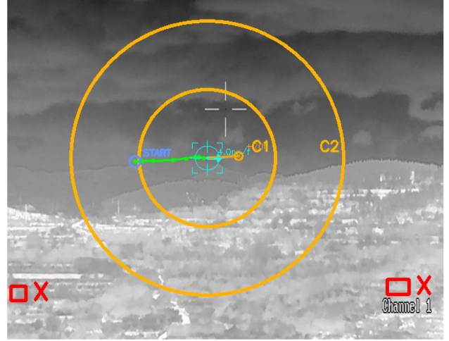
Figure 3. Temporal-coherence filtering in an operational thermal scene. The true UAV track remains consistent with the predicted path, while thermally salient but motion-incoherent false alarms are rejected.
